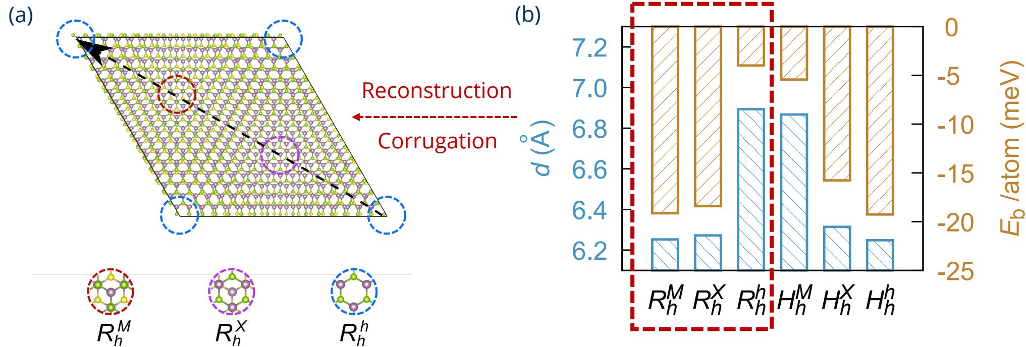
(a) 3 high-symmetry stackings and transition stacking regions. (b) Interlayer distance and binding energy of corresponding high-symmetry stackings.
