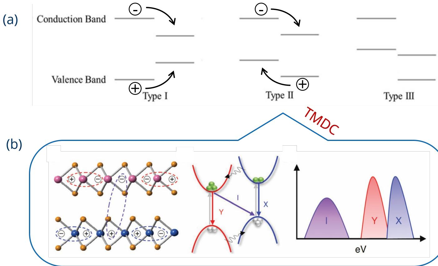
(a) Different types of vdWH band structures.<sup>[1]</sup> (b) Excitonic behavior in Type-II alignment vdWH.<sup>[2]</sup>
